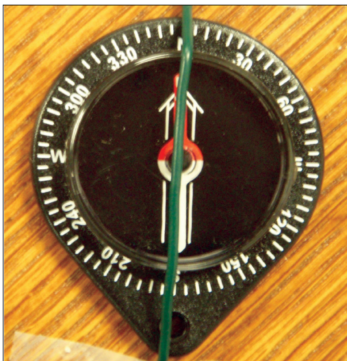
Fig. 2. With no current in the wire, the compass points north.
