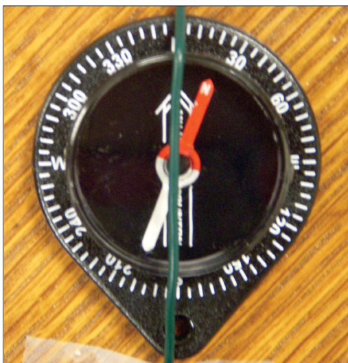
Fig. 3. When 0.314 A is run through the wire, the compass deflects by approximately 20°.
